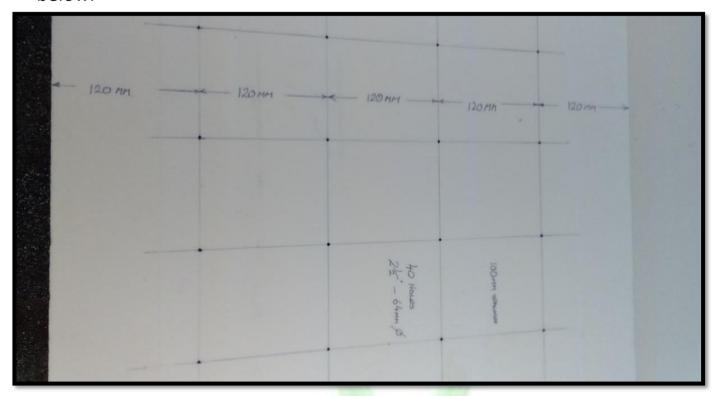
2. Mark out 4 rope holes, 1 in each corner, 75mm in from corner. See below
